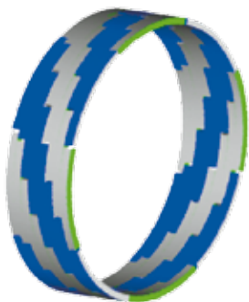
Schematic picture of LOC-technology providing fiber orientation and stretch-ability
